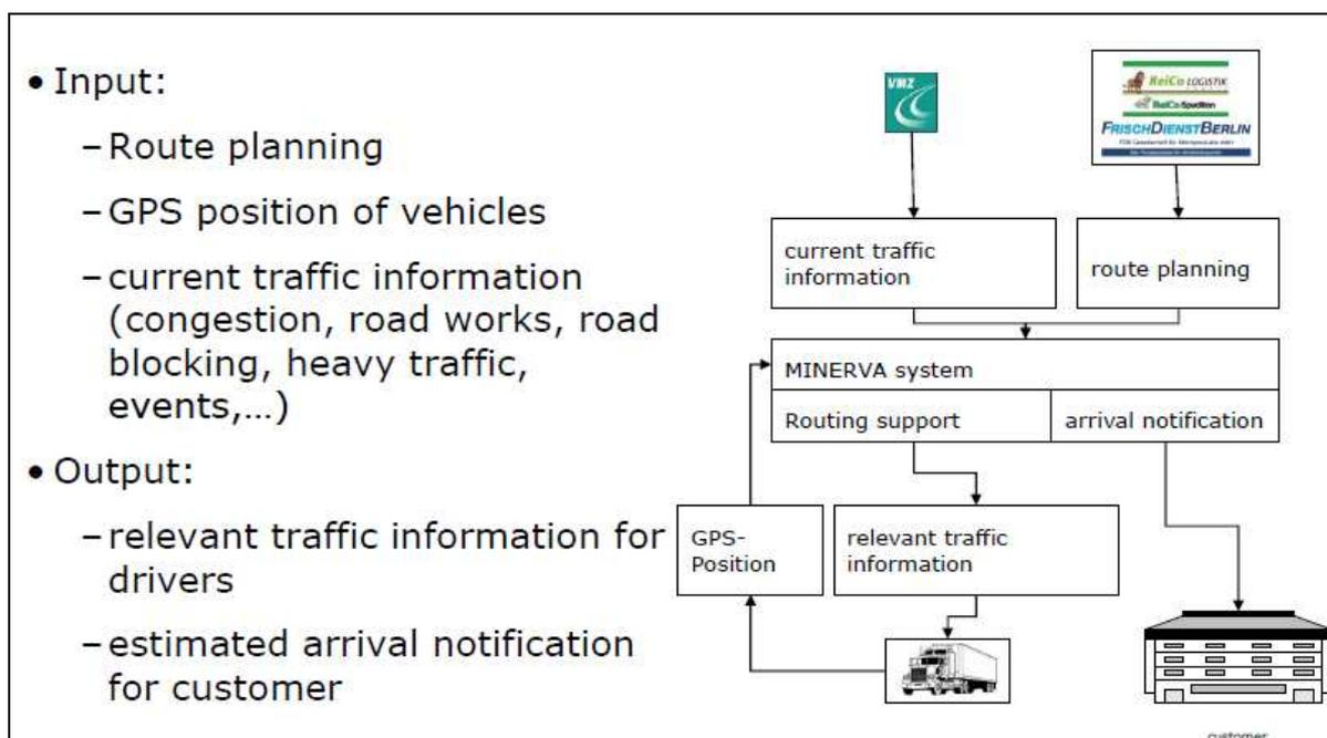
Fig. 2. Components and data flow of the MINERVA system
