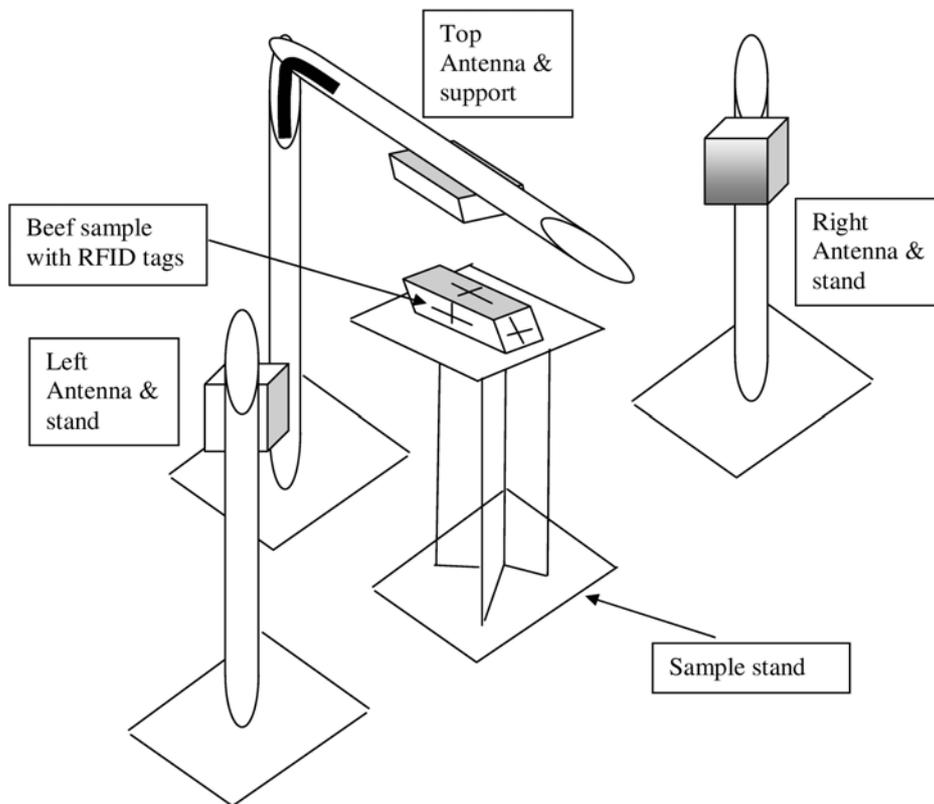
Fig. 3. Schematic representation of the physical arrangement of RFID readability test apparatus (this study).
