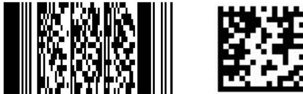
Fig. 2. The word "traceability" encoded in PDF417 (left) and Data Matrix (right) Codes.
