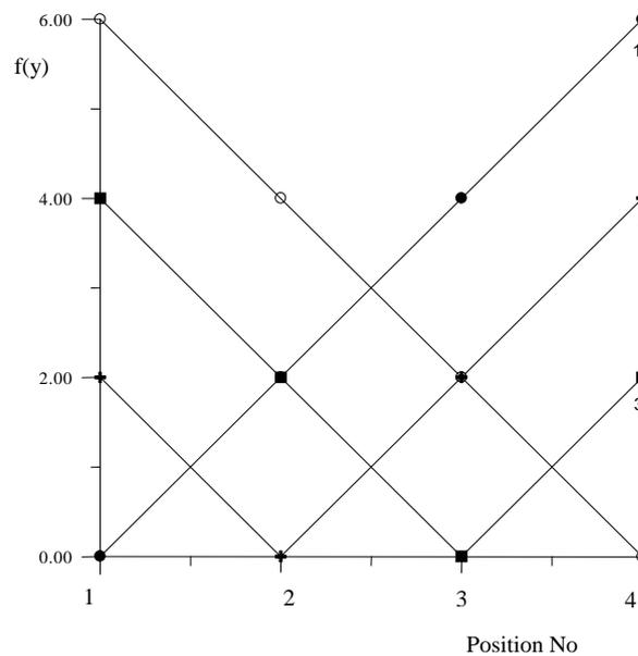
Fig. 2. The diagram of the dependence of the stop spots of the AGV on the route covered in the time of service of  $M=4$  assembly cells. The AGV stop at the cell: 1 – first, 2 – second, 3 – third, 4 – fourth.
