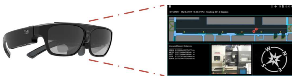
Fig. 2. Presentation of information with Smart Glasses (ODG R-7, real screenshot of Smart Glasses on right).
