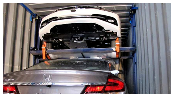
Fig. 6. Visible elements of rack construction with possibility of height regulation
