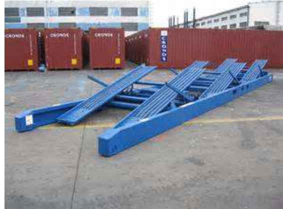
Fig. 2. Flat pallets with tippable rack for fastening of transported cars
