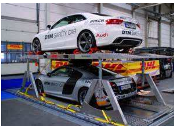
Fig. 1. The variant of possible stacking based on construction of flat transport pallets
