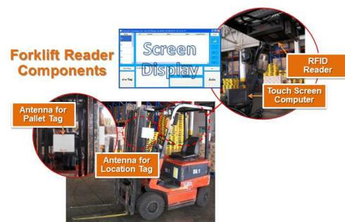
Fig. 8. Reader which mounted on the Forklift truck
