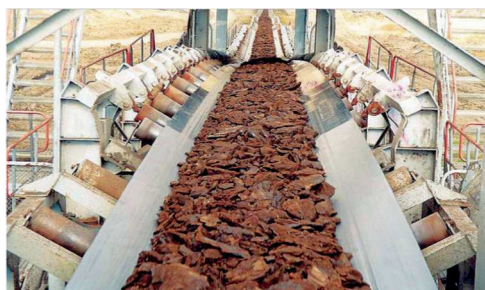
Fig. 1. The technological transport of lignite opencast mine (conveyor belt)
